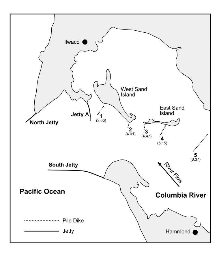
**Figure 2.** Location of pile dikes in the lower Columbia River (near the mouth of the river). The river mile for each pile dike is shown in parentheses under the dike number.
