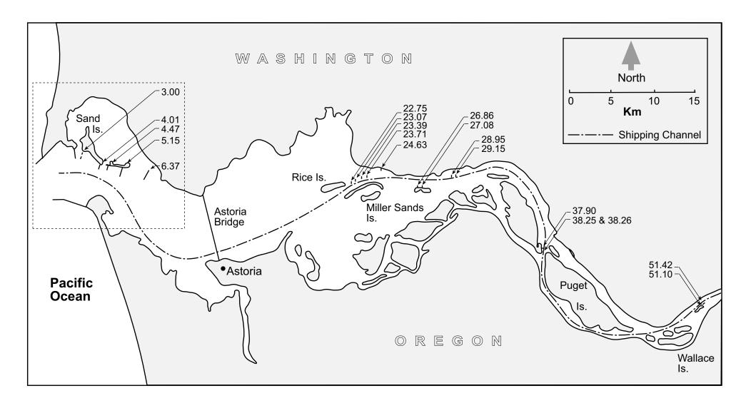
**Figure 1.** Location of pile dikes (in river miles) and the shipping channel (dashed line) in the Columbia River Estuary. Area within the dashed line box is shown in greater detail in Figure 2.
